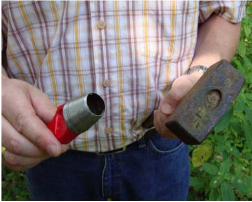
Figure 3a: Punch and hammer for cambium collection
