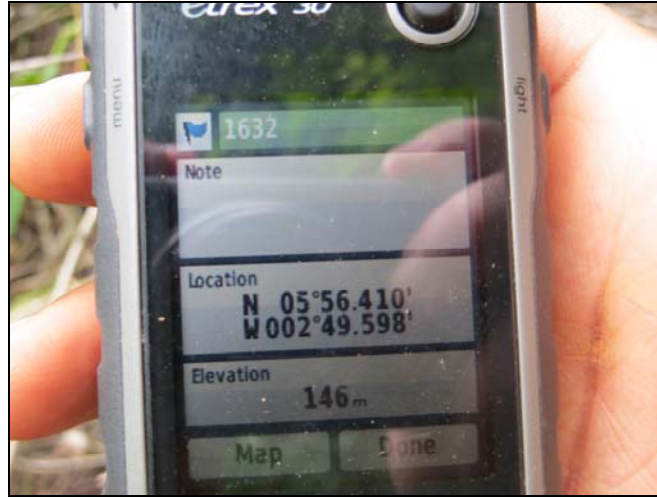
Figure 2: Use the GPS to measure longitude and latitude in decimal degrees and the altitude (elevation) in meters
